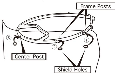
2. While holding the frame and center post with 2 fingers, attach the other side of shield holes by pushing over side posts ④ and ⑤. (Pulling the edge of the shield a little while attaching makes it easier) Ensure that all 5 posts of frame are attached securely to the shield.
