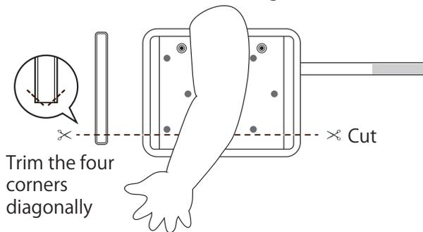
**2** Turn over the wrap and attach the white Velcro loop strip and the stabilizing stay to the cut side of the cardboard wrap.
